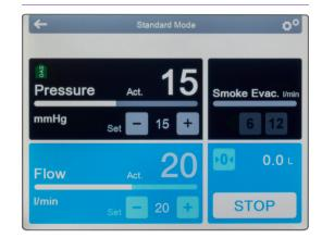
The Insufflator has a 5.7" touchscreen with intuitive operating concept. Additionally the device offers an integrated smoke evacuation and an optional gas heating function.
